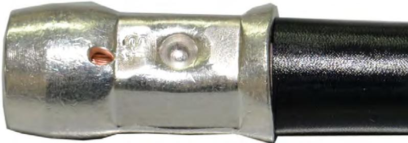
Not correctly crimped.
