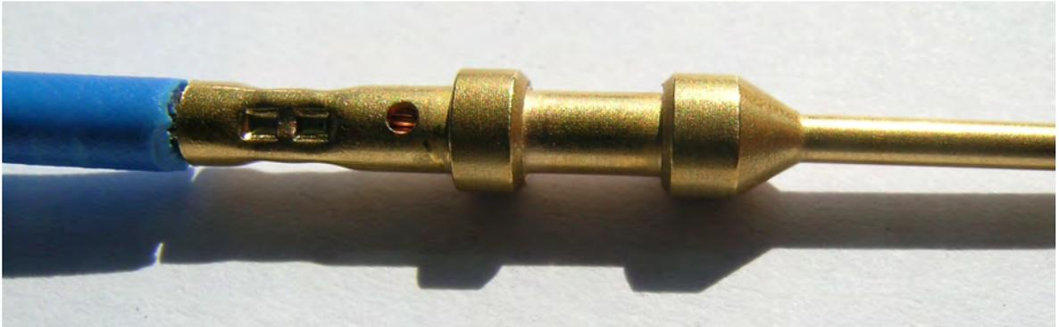
Not correctly crimped.
