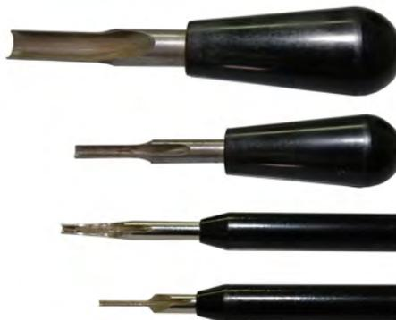
The individual wire is, as shown in the picture, placed in the half-shell of the installation tool and pushed from the cable side, as far as it will go, into the correct hole of the rubber mount (pay attention to plan).
