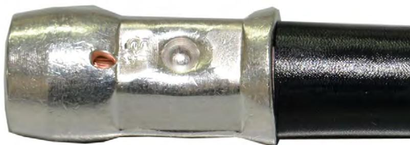
Not correctly crimped.
