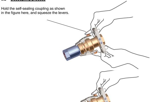
As soon as the levers are free of the adaptor, the coupling can be removed.
