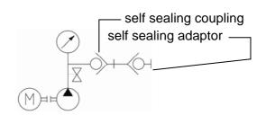
Test 2: self sealing coupling disconnected
